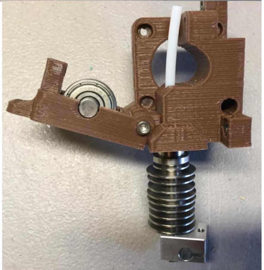
Next we will cut the PTFE Tube so its goes just past the extruder block, make sure you push the hot end as far into the extruder block as possible before cutting the ptfе tube. Now you can remove the hot end and we will install it later.
