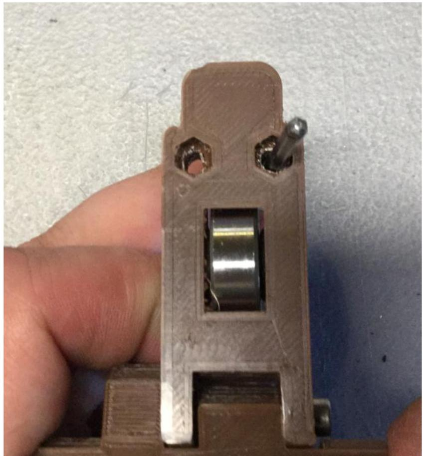
**Install two M4 nuts in the nut traps shown by the Red Arrows**
