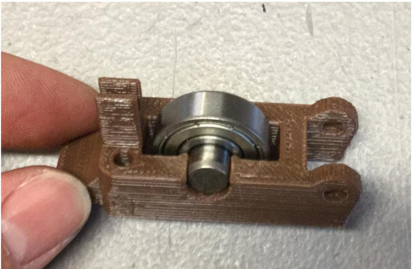
**Install the Guidler onto the extruder block and secure using the M3x30mm bolt and regular M3 nut as shown below.**
